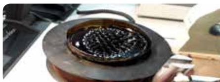
Magnetic liquids resemble Hedgehogs in strong magnetic fields – but their properties are useful in shock absorbers!
